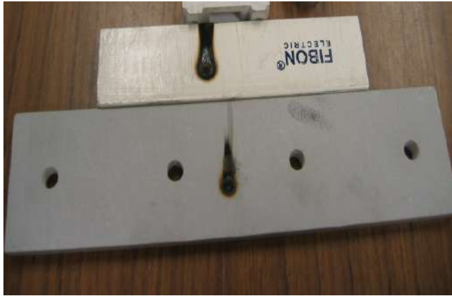
4.1a Insulation materials subjected to glow-wire test at 960°C.
