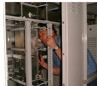
4.7d A testing engineer checking the integrity of the busbar system after short-circuit withstand test of Series Forti LV System.
