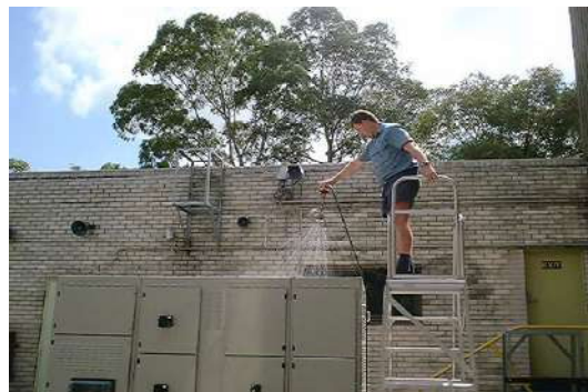
4.2b IP X4 in progress
