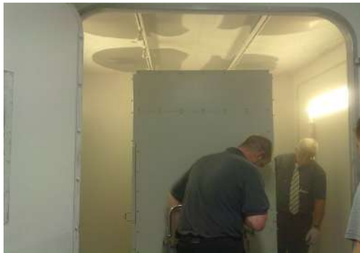
4.2a A panel in a dust chamber preparing for IP5X test
