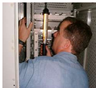
4.7d A testing engineer checking the integrity of the busbar system after short-circuit withstand test of Series Forti LV System.
